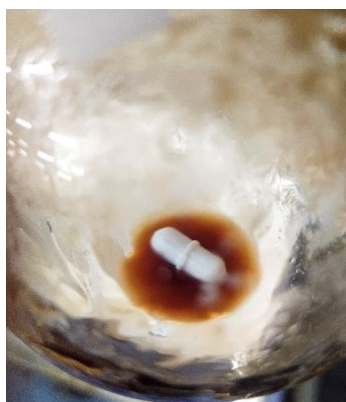
Figure 4. The initial appearance of the DES mixture which turned into a homogeneous brown liquid during heating
